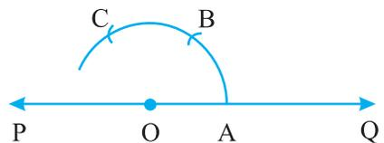
**Step 5** Join OC,  $\angle COA$  is the required angle whose measure is  $120^\circ$ .
