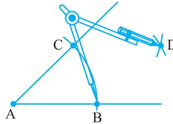
**Step 3** With the same radius and with C as centre, draw another arc in the interior of  $\angle A$ . Let the two arcs intersect at D. Then  $\overline{AD}$  is the required bisector of  $\angle A$ .
