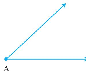
**Step 1** With A as centre and using compasses, draw an arc that cuts both rays of  $\angle A$ . Label the points of intersection as B and C.
