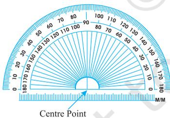
A semi-circular device graduated into 180 degree-parts. The measure starts from  $0^\circ$  on the right hand side and ends with  $180^\circ$  on the left hand side and vice-versa.
