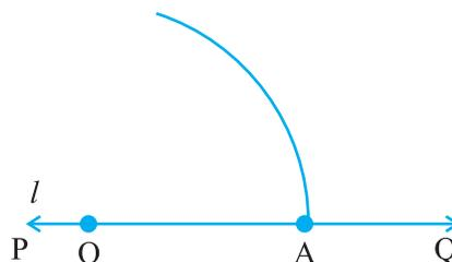
**Step 3** With the pointer at A (as centre), now draw an arc that passes through O.
